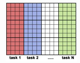
After the array is distributed, each task executes the portion of the loop corresponding to the data it owns. For example,
